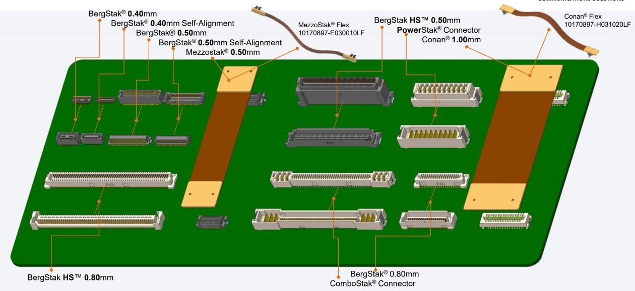
Broad offering of Board to Board Connectors to support various customer needs for Flexible Printed Circuit assembly.
