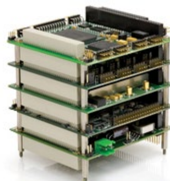
PC/104 stack with CPU, Power Supply and Peripheral Modules. The stack is assembled with PC/104 stand-offs creating a singular and rugged unit.
