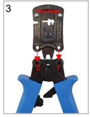
Open the handles and insert the tool head into the open holes. The laser marking of
