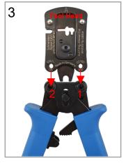
Open the handles and insert the tool head into the open holes.
