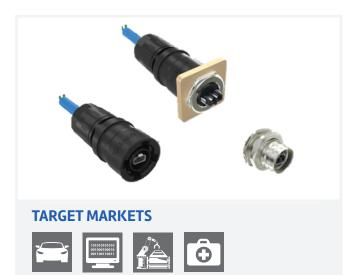
Amphenol's IP67 rated SPE connectors have a circular M12 size form factor with push-pull positive latching. Robust panel-mount receptacles are available with right angle and vertical PCB tails or solder cups for discrete wire termination. When mated with the field terminable plugs, a completely sealed, shielded interface is provided, rated up to 4A supporting PoDL (Power over Data Link) up to 1km when using 18AWG single pair cable.
