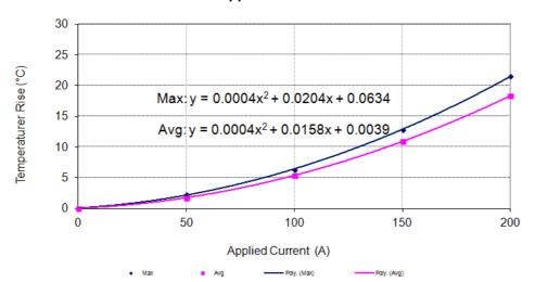
Above rating is for reference only. Appropriate de-rating is required per ambient conditions, bus bar size to achieve thermal balance, gross heating from adjacent components, and other factors that influence connector performance.
