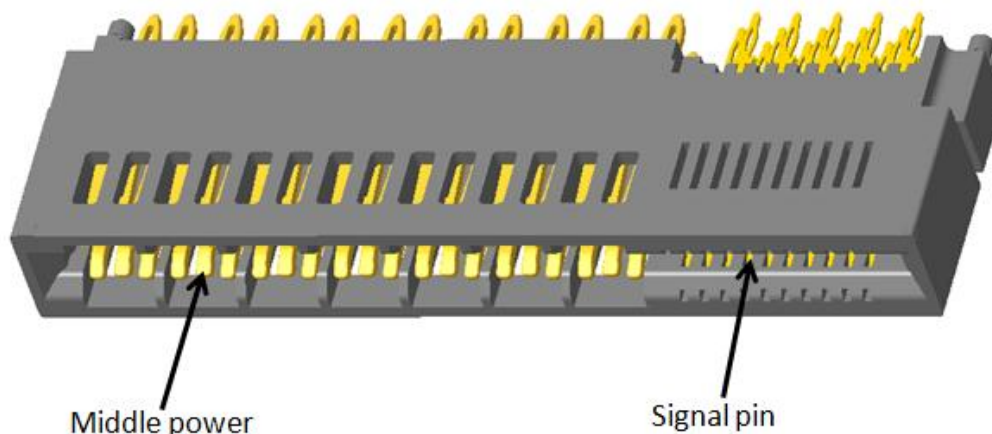
Configuration 14 Middle power + 20 Signal as shown (One Middle power has three contact beams and two tails)
