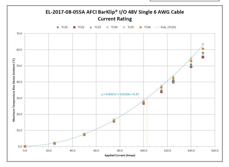
Notes: Above rating is for reference only. Appropriate de-rating is required per ambient conditions, bus bar size to achieve thermal balance, gross heating from adjacent components, and other factors that influence connector performance.
