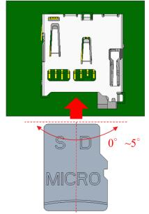
Horizontal insertion angle:  $0^{\circ} \sim 5^{\circ}$
