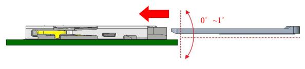
Vertical insertion angle:  $0^{\circ} \sim 1^{\circ}$
