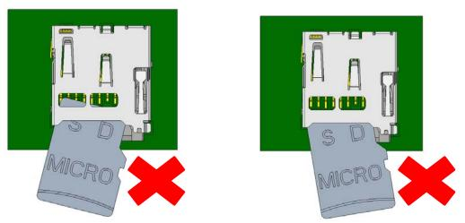
The horizontal inclination angle cannot be greater than  $5^{\circ}$
