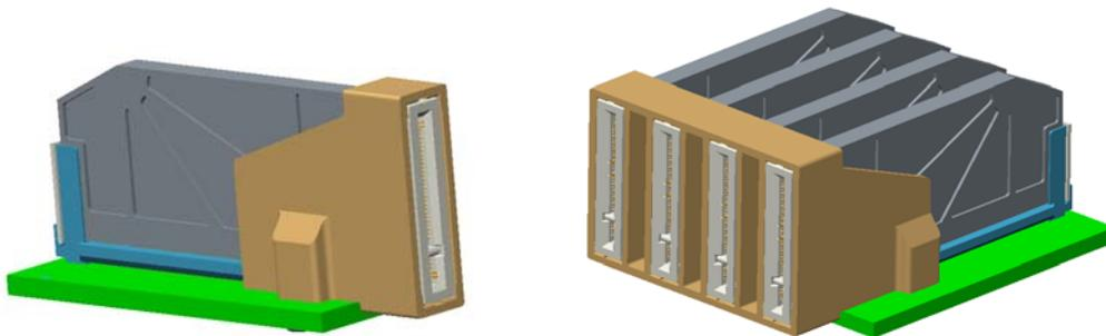
**Figure 1: Orthogonal NF1/NGSFF Connectors**
