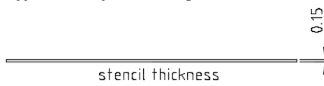
Figure 9: RECOMMENDED STENCIL THICKNESS REQUIREMENT (YOUR CONFIGURATION MAY VARY)
