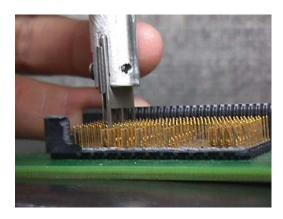
Step 2 Slide shield extraction tool over damaged shield, making sure shield is inserted between extractor claw and protective cover plate.
