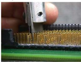
Step 3 Insert the claws into the chevron knockout areas of the damaged shield.
