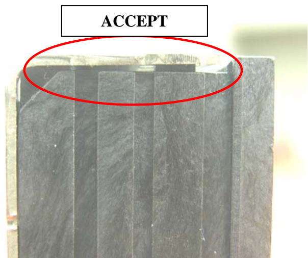
Figure 8.63. VHDM alignment tabs partially protruding. Figure 8.65. VHDM alignment tabs partially protruding.
