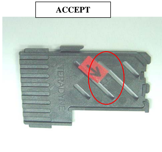
Figure 8.53. Cracked body of 8 Row VHDM endcap
