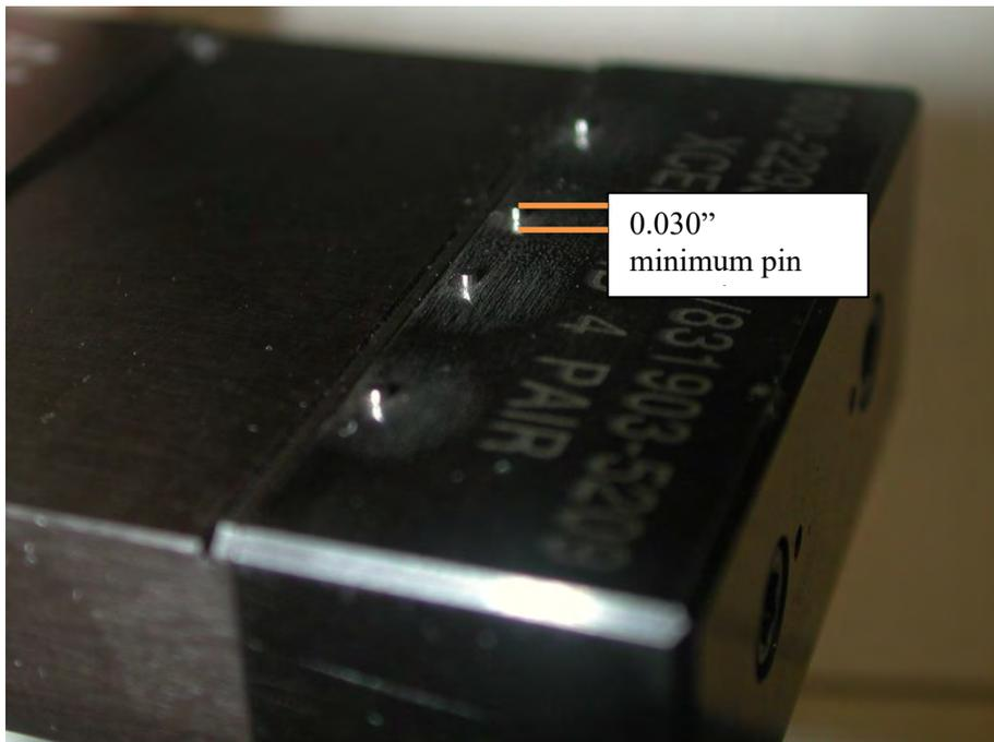
Figure 1: Stiffener removal pins protruding out the bottom of the pin block
