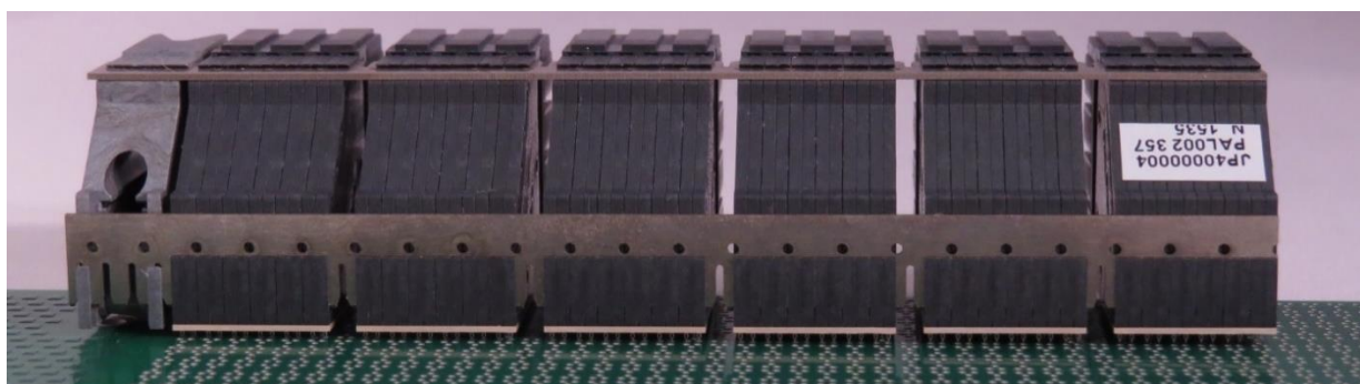
Figure 5: Rear view of the assembly. Check for bent pins.
