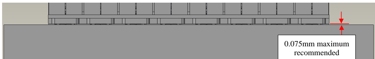
Figure 9: 0.075mm maximum height off board surface (rear view)
