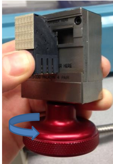
Figure 20. Top Stiffener Installation (Loose Connector)
