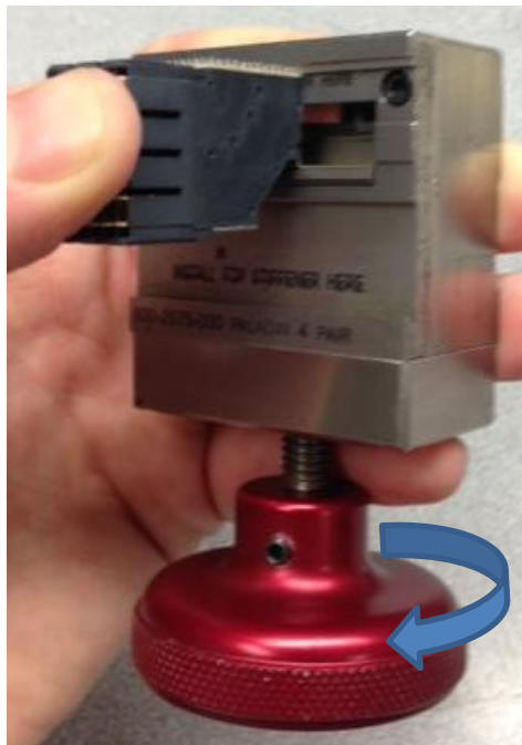
Figure 21. Back Stiffener Installation (Loose Connector)
