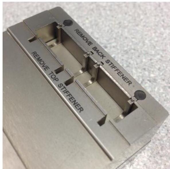
Figure 2. Pin locations for RAF back stiffener removal
