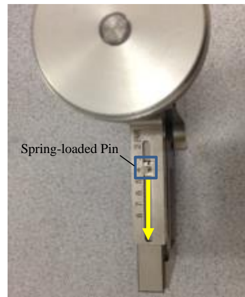
Figure 13. Paladin RAF Module Removal Tool Spring Loaded Pin.
