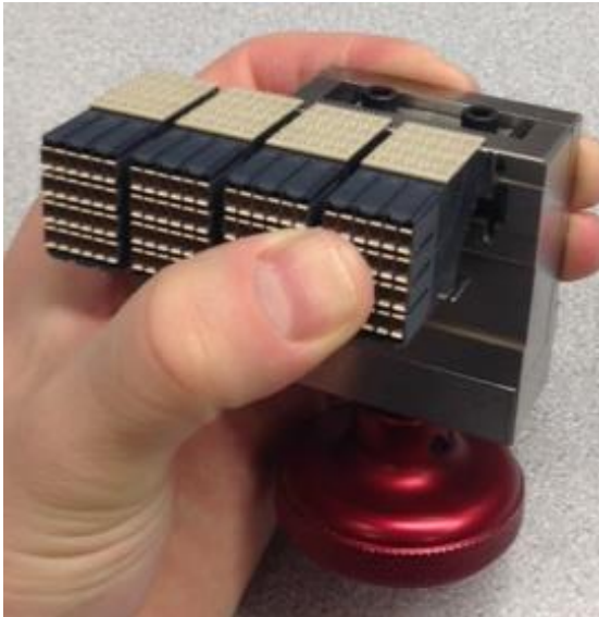
Figure 8. Back stiffener removal on loose Paladin RAF connectors greater than 2" in overall length (50.8mm)
