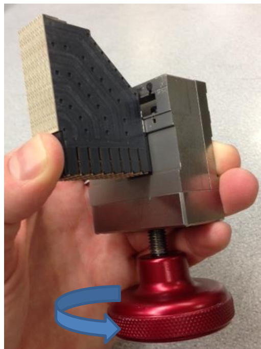
Figure 6. RAF Top Stiffener Removal on Loose Connector
