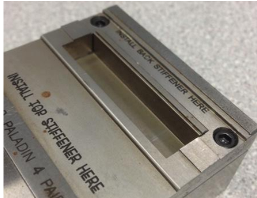
Figure 19. Jaw location for RAF top stiffener installation
