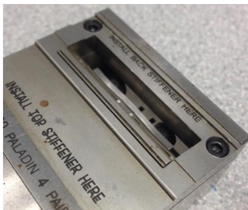
Figure 18. Jaw location for RAF back stiffener installation
