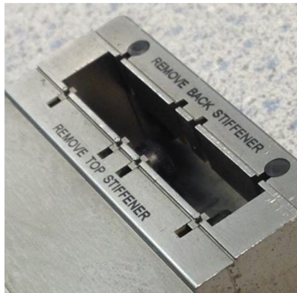
Figure 3. Pin locations for RAF top stiffener removal
