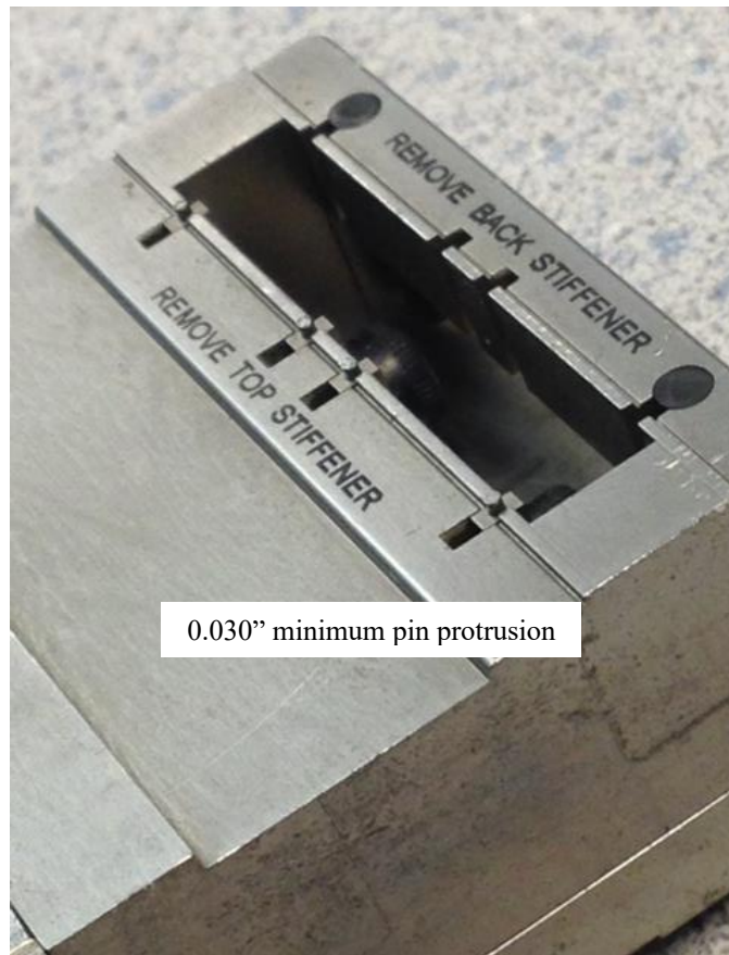
Figure 1: Stiffener removal pins protruding from the bottom of the pin block.
