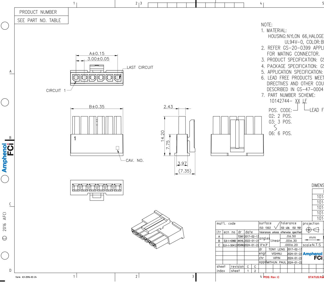
HOUSING: NYLON 66, HALOGEN FREE UL94V-0, COLOR: BLACK 2. REFER GS-20-0399 APPLICATION SPECIFICATION 3. PRODUCT SPECIFICATION: GS-12-1291. 4. PACKAGE SPECIFICATION: GS-14-2419 (BULK PACKED) 5. APPLICATION SPECIFICATION: GS-20-0399. 6. LEAD FREE PRODUCTS MEET EUROPEAN UNION DIRECTIVES AND OTHER COUNTRY REGULATIONS AS LEAD FREE
